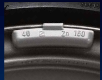
Coated weights: Sealed epoxy finish. At least 0.1 mm thick. Approx. 5% aluminium pigments, embedded in synthetic molecules. The result: no oxidation of surface.
