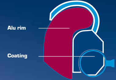
Coated weights: Sealed epoxy finish. At least 0.1 mm thick. Approx. 5% aluminium pigments, embedded in synthetic molecules. The result: no oxidation of surface.
