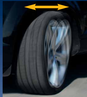
Dynamic imbalance: The wheel has a tendency to wobble.
