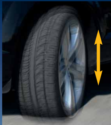
Static imbalance: The wheel has a tendency to jump.
